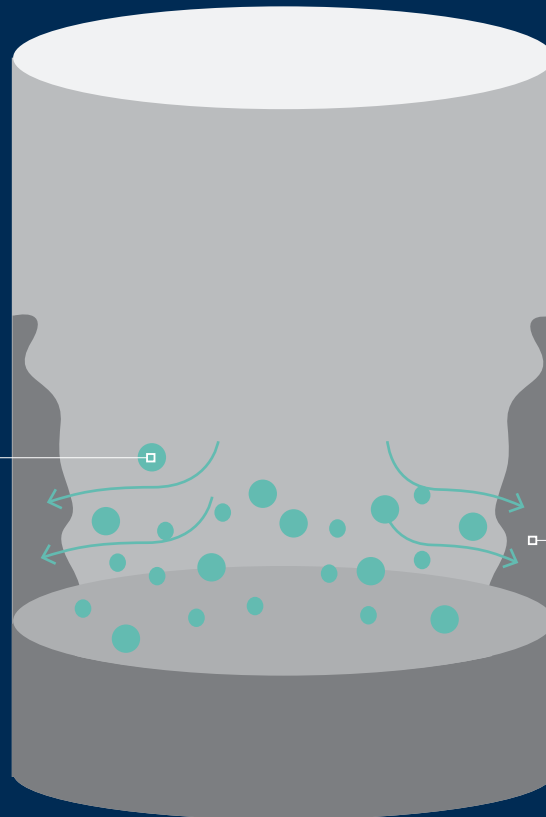
Figure 1. At temperatures above approximately 70°C, the water from gypsum/wet materials moves to the colder parts of the silo (typically the wall, silo outlets and roof), where it prehydrates the cement and eventually forms coating and lumps.
