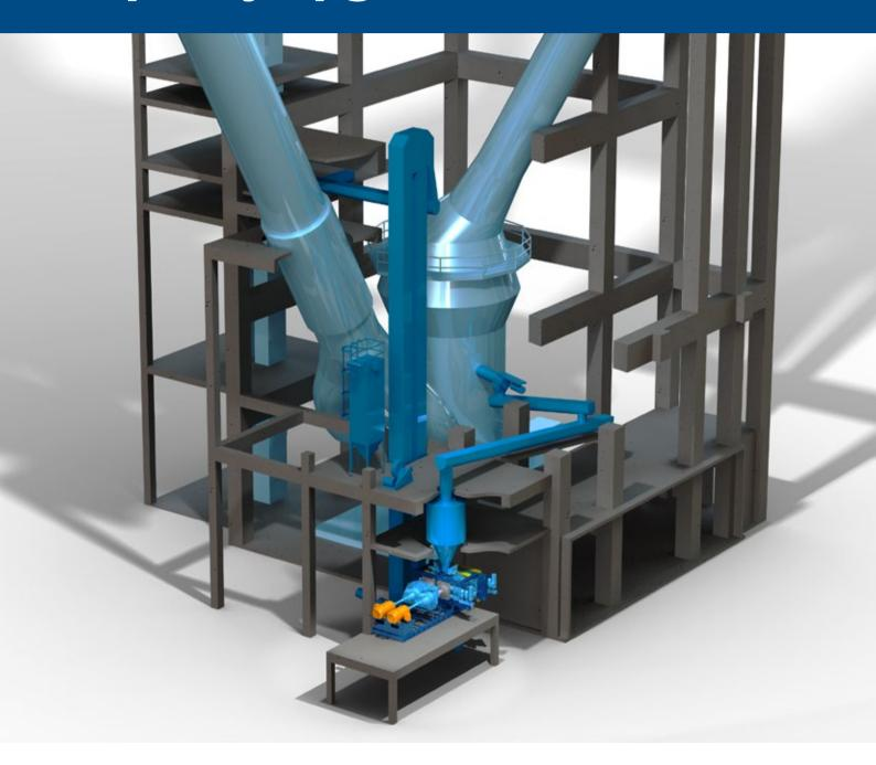
Now it's possible to increase the capacity of a vertical roller mill by up to 15%. Simply integrate a specially adapted Hydraulic Roller Press (HRP) to boost output.
