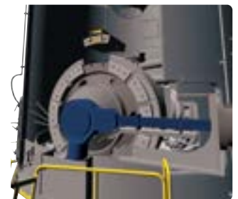
Easy changing of the wear segments in larger mills.
