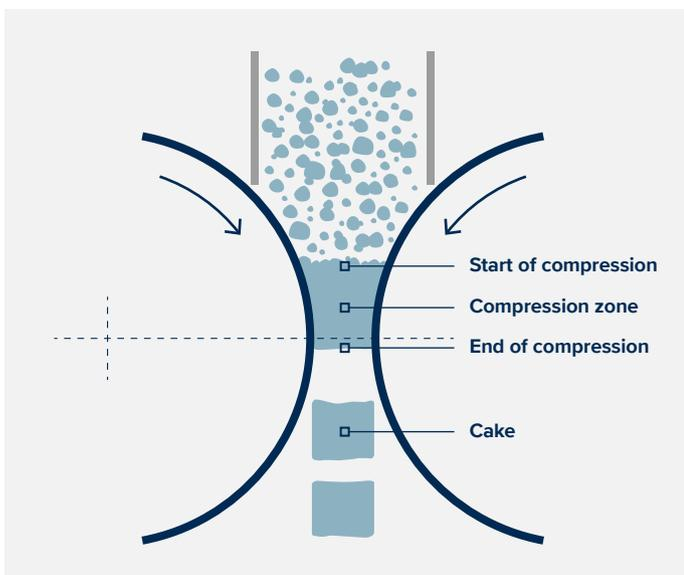
The figure shows how feed material is exposed to a very high pressure in the HRP.
