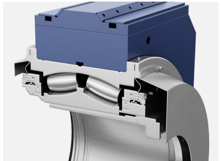
The oil-cooled spherical bearings.
