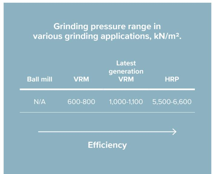
As shown on the figure, the HRP is the most efficient machine amongst all grinding machines.
