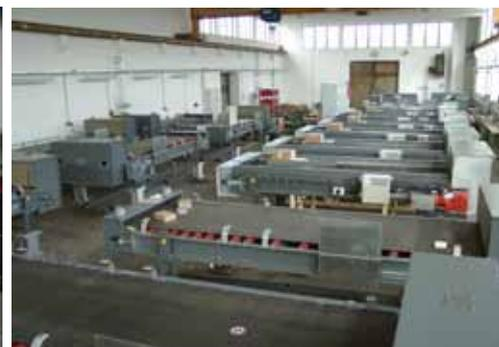
*FLSmidth Pfister assembles all weighfeeders in Augsburg/Germany and in India*
