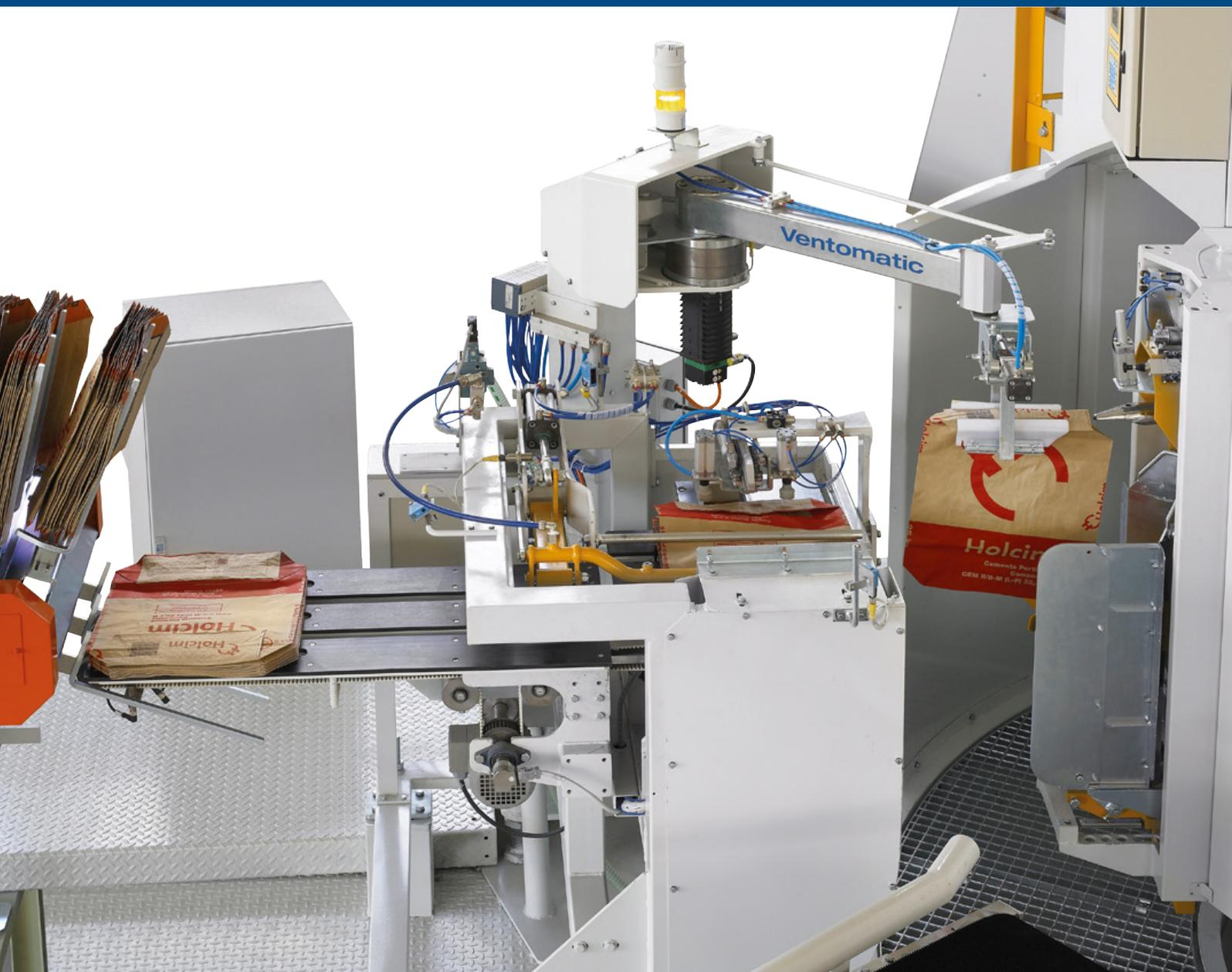
FLSmidth Ventomatic SpA offers a complete range of machines for the empty bags handling and placing empty valve bags onto in line and rotary packers.
