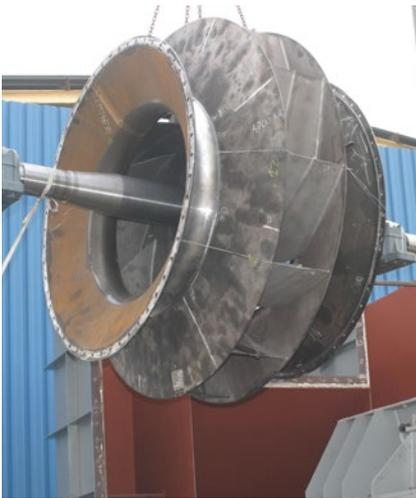
*Impeller, delivered pre-assembled*
