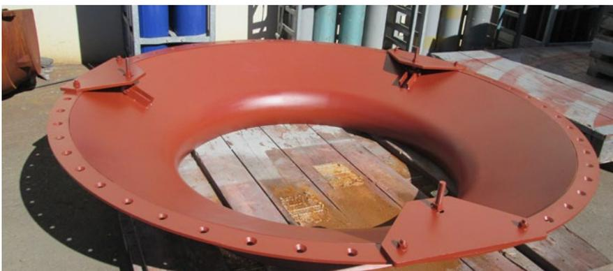
*Tool for easy adjustment of inlet cone*
