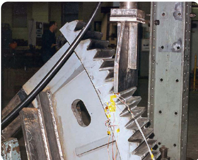
Load testing: a fabricated gear undergoes rigorous evaluation at Lehigh University
